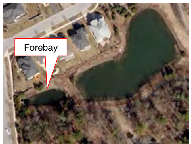
Example of a Quality Control Pond
