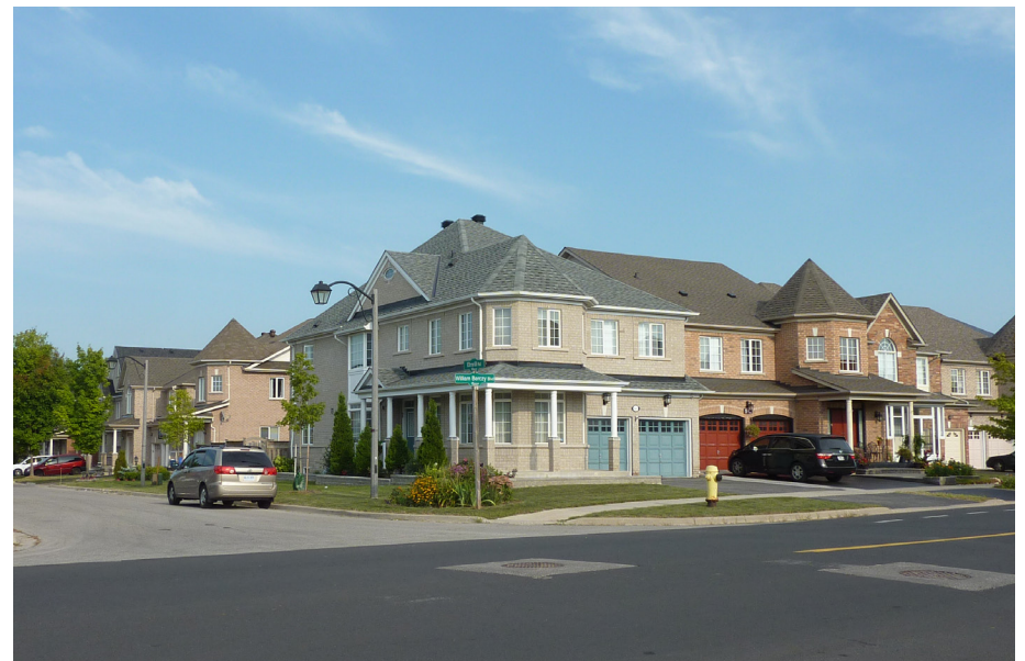
Cap end block configurations increase active frontages on the public realm and visually shorten the block.
